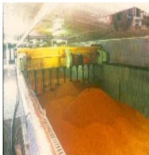
Figure 6 Industrial sorghum maltings in southern Africa. A) Outdoor floor maltings, B) Pneumatic maltings
